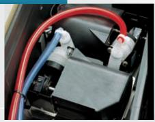
Belows pumps ensure the greatest possible replenishment accuracy - electronically calibrated for long, trouble-free service.
