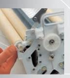
Practical snap-lock bearings eliminate the need for special tools when removing rollers for faster and easier maintenance.
