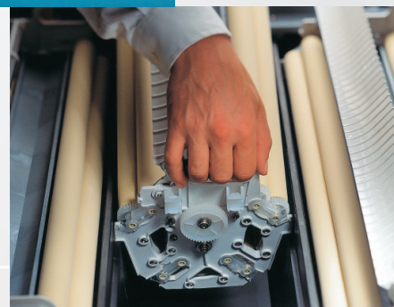
Rack-mounted modules make it easy to disassemble a machine for maintenance.
