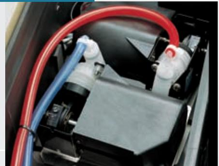
*Belows pumps ensure the greatest possible replenishment accuracy - electronically calibrated for long, trouble-free service.*
