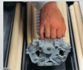
*Rack mounted modules make it easy to disassemble the machine for maintenance.*
