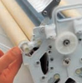
*Practical snap-lock bearings eliminate the need for special tools when removing rollers for faster and easier maintenance.*
