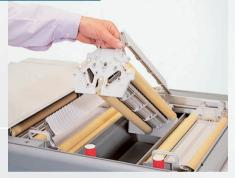
All rollers are located in racks. Rollers in wet sections are easily removed, without tools, for cleaning or service purposes.
