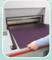
Easy Operation – Operators simply slide in a plate that has been notched for your press, matching it to the Mako 4 pin bar system. They then release the file with the touch of a button and the Mako 4 does the rest. The file will be imaged and the plate is delivered directly to an online processor. This process makes the Mako 4 as easy to use as a contact frame.
